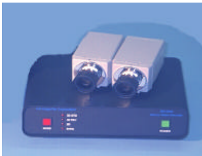
3-D (field-sequential) video Encoder and Decoder combined into one box. (Cameras optional)
