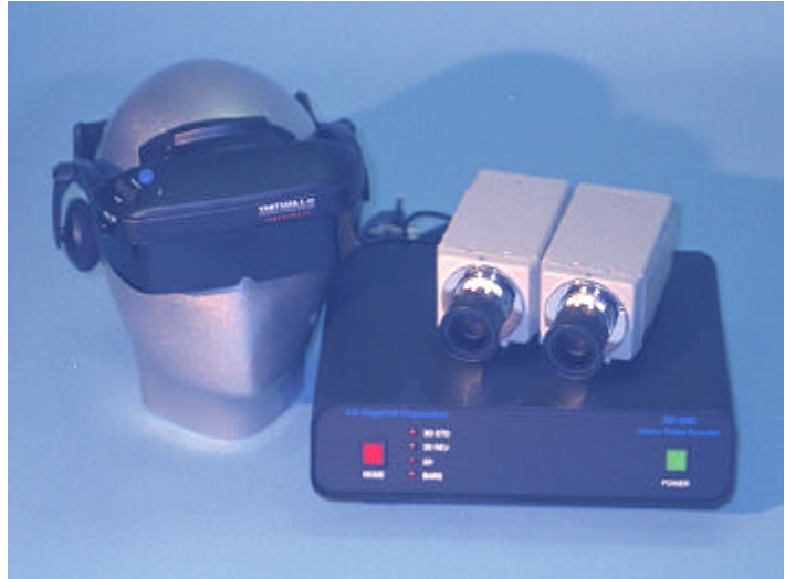
Stereoscopic 3-D Video Encoder (Cameras and HMD optional)
